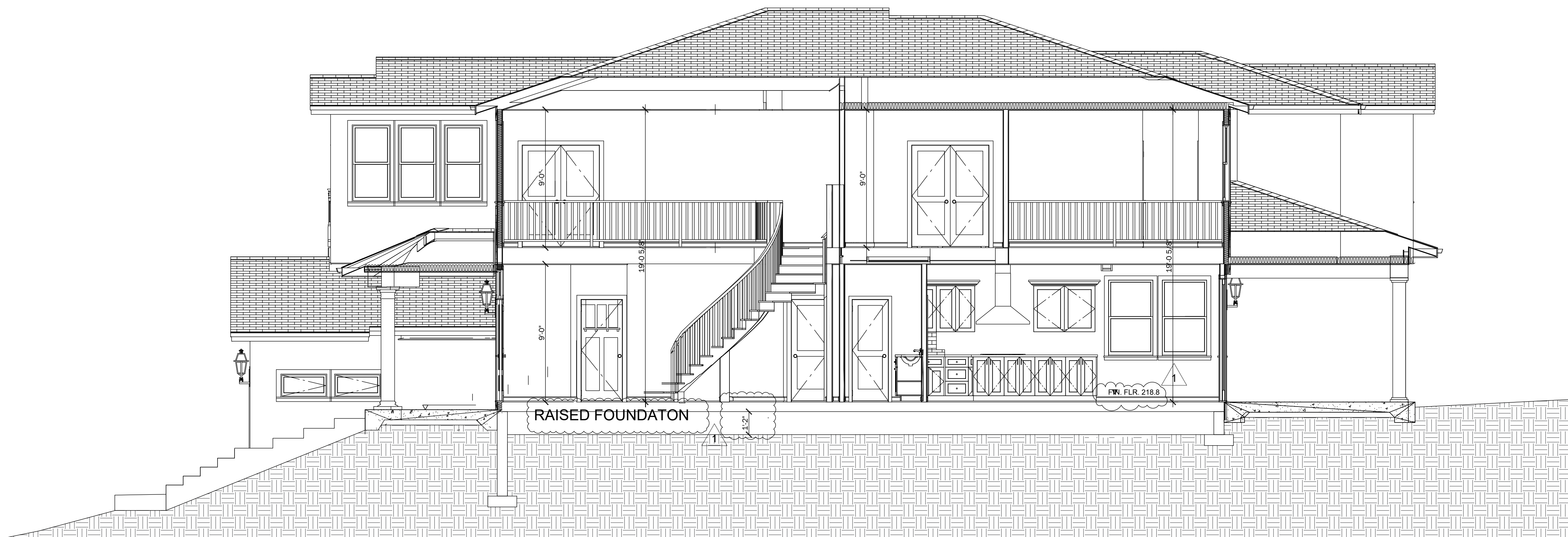
1 LONGITUDINAL BUILDING SECTIONS SCALE: 1/4"=1'-0"
