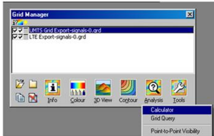
Figure 44 : Launching the Vertical Mapper Grid Calculator
